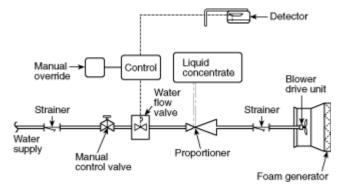
(a) *Foam Generators* — *Aspirator Type.* Foam generators can be fixed or portable. Jet streams of foam solution aspirate sufficient amounts of air that is then entrained on the screens to produce foam. *[See Figure A-1-9.5(a).]* These generators usually produce foam with expansion ratios of not more than 250:1.
