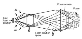
(b) *Foam Generators* — *Blower Type*. Foam generators can be fixed or portable. The foam solution is discharged as a spray onto screens through which an airstream developed by a fan or blower is passing. The blower can be powered by electric motors, internal combustion engines, air, gas, or hydraulic motors or water motors. The water motors are usually powered by foam solution. *[See Figure A-1-9.5(b).]*
