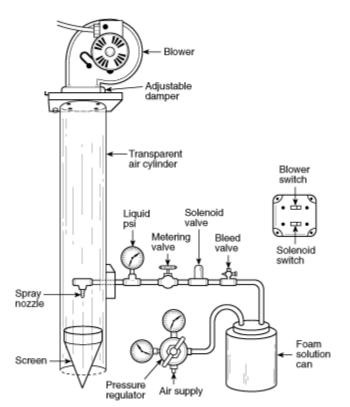
Figure A-1-10.5(b)(2) Typical drainage drum for high-expansion foam expansion and drainage test.
